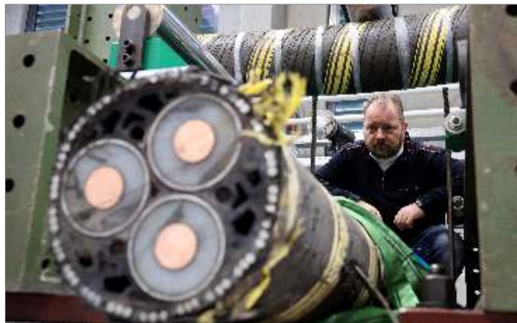
Martin Radtke, technician, squats at a test stand for submarine cables in the new research hall of the Faculty of Mechanical and Marine Engineering at the University of Rostock, Germany.
